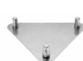
BASE 20D weight = 0,740 kg Baseplate for E20D truss incl: CCS4-402 | Offset half conical coupler BM-M6x020-IB-CS | Bot M6x20mm countersunk
